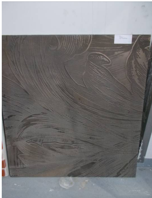
Plate 1 - Before and After Weathering of the Jesmonite GRC Grade 18. Metallic Panel
